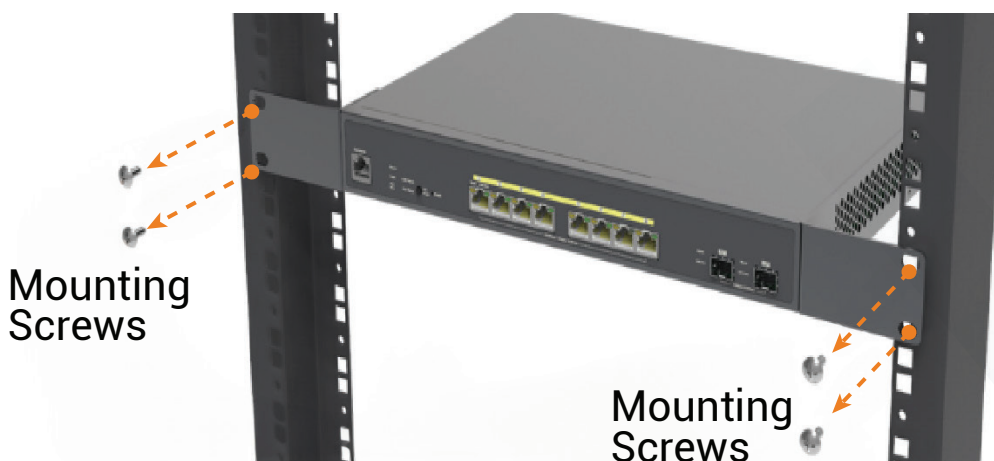
Installing the switch in a Rack
